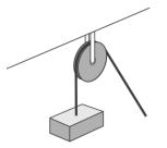
Pulleys can be used to make a small force lift a heavy load.
