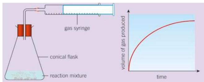
In this case, the volume of gas formed is collected in the syringe.
