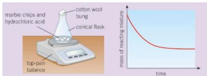
In this case, the mass decreases as a gas ( $\text{CO}_2$ ) is formed and escapes the conical flask. The cotton wool is to stop the solution escaping.
